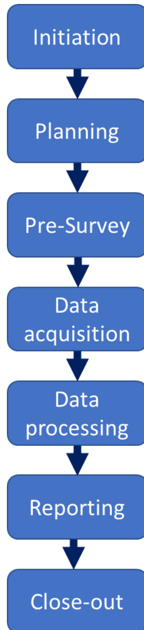
Figure 2: Process flow for power performance assessment of marine energy devices
