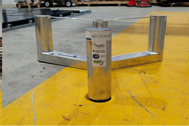
Figure 45. Model with tower removed (FSS).
