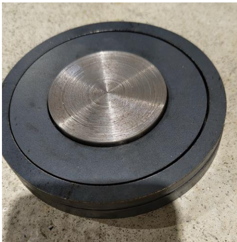
Figure 46. Ballast weights stack.
