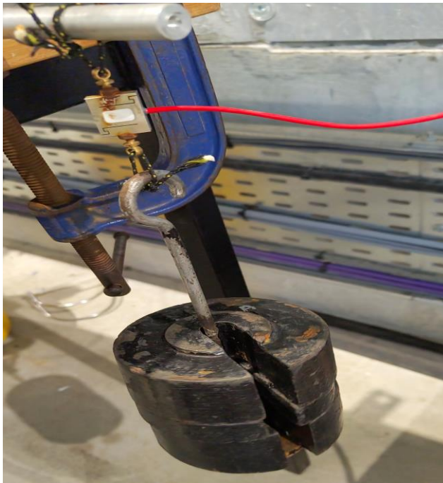
Figure 50. Futek load cell during calibration process.
