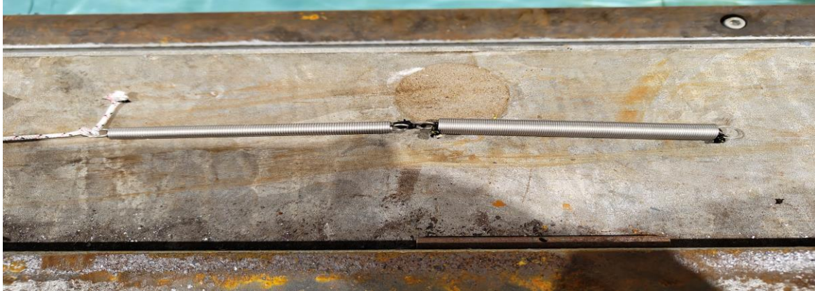
Figure 53. Spring setup used for mooring lines in the DOB.
