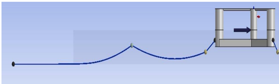
Figure 37. Early iteration of DEA mooring system for Bantry Bay.
